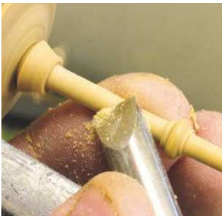
▲ Pic.25 Please make sure that your fingers are underneath the toolrest when supporting your work like this. Work the finial down in stages, cutting in the direction of the chuck
